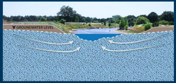
High Groundwater Levels Groundwater Maintains Stream Flow
