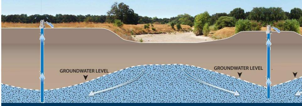
Pumping Lowers Groundwater Levels Stream Loses Flow to Groundwater
